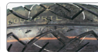
Mouse bites Because of tire store improper, tire was bitten by the mice
