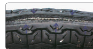
Tread cut wounds Tire surface cut wounds by external things
