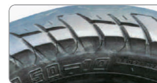
Tire shoulder pattern cracked Tires running with low air pressure long time, killing tire shoulder pattern parts and tire, cause tire shoulder cracked.
