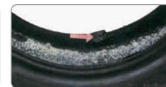
Tire lip lesion (by pry bars) Improper operation when tires and rims assembly, causing tire labial ministry picked great damage
