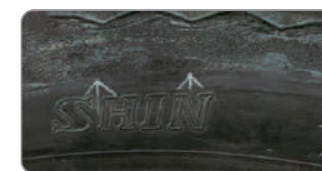
Tire shoulder pattern cracked Tires running with low air pressure long time, killing tire shoulder pattern parts and tire, cause tire shoulder cracked.
