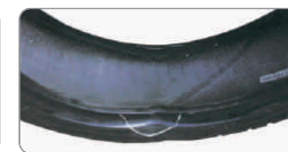
Tire lip damage bending Tires lip bending were caused by external extrusion
