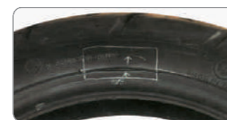
Yarn was breaking by slams (out) When tire in low air pressure condition go through the pavement dent or obstacles, tires bear thumping excessive force, causing tire body cotton/yarn was cut off by the wheel rim.
